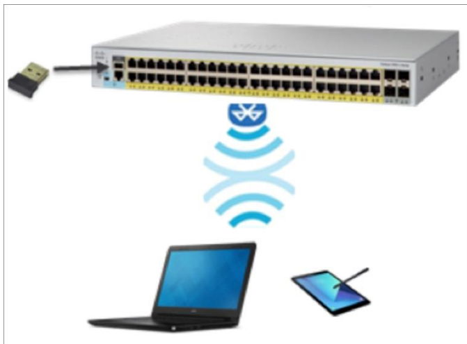
Figure 2. Over-the-air switch access using Bluetooth
