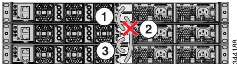
In this figure, StackPower port B on the center switch has failed and this stack partitions into two stacks. The top two switches share power, and the bottom switch is now a separate stack.
