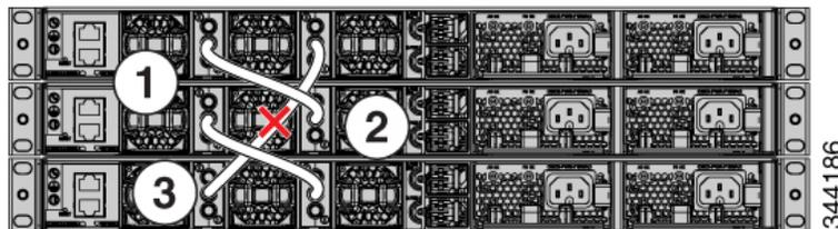
In this figure, link 2 is bad. Therefore, this stack partitions into two stacks, and the top and bottom switches become the active switch in the stack. If the bottom switch is a member (not active or standby switch), it reloads.
