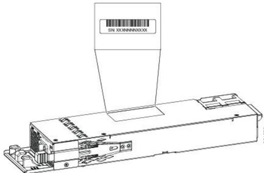
**Figure 35: 715-W and 350-W AC Power Supply Serial Number**
