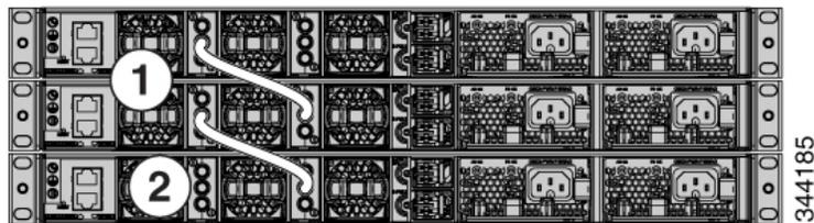
The figures below show data stacks of switches with failover conditions. In this figure, the StackWise cable is bad in link 2. Therefore, this stack provides only half bandwidth and does not have redundant connections.
