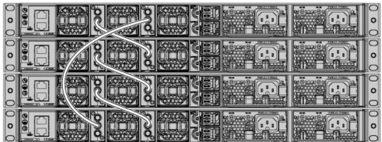
This example shows a recommended configuration when the switches are mounted side-by-side. Use the 1-meter and the 3-meter StackWise cables to connect the switches. This configuration provides redundant connections.
