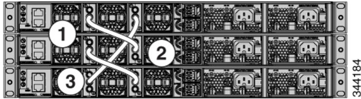
This figure shows an example of a stack of switches with incomplete StackWise cabling connections. This stack provides only half bandwidth and does not have redundant connections.
